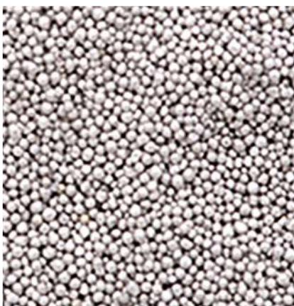
**Figure 3: Ultrasoft Shot, metallurgically enhanced soft steel media**
