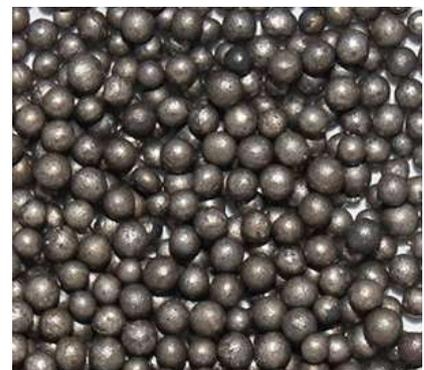
**Figure 2: Low-Carbon Cast Steel Shot**
